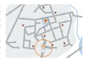
Metered Areas (DMAs). Technolog's advanced algorithm analyses and learns from the DMA's pressure and flow data to identify network anomalies and localise the position within the DMA. Potential leaks are presented to the user within the same feature rich user interface and visualised as hotspots on a map viewer.
