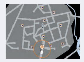
LEAK's state of the art algorithm analyses the deviation from the group's learned pressure relationships and benchmark to highlight the logger nearest to the network anomaly.
