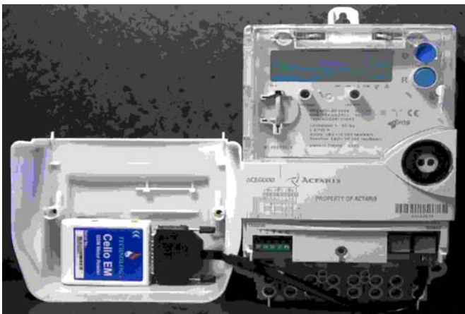
Above is shown an Actaris ACE6000 meter fitted with a Cello EM via an interface adapter cable. See last page for examples of meters to which Cello EM can connect.
